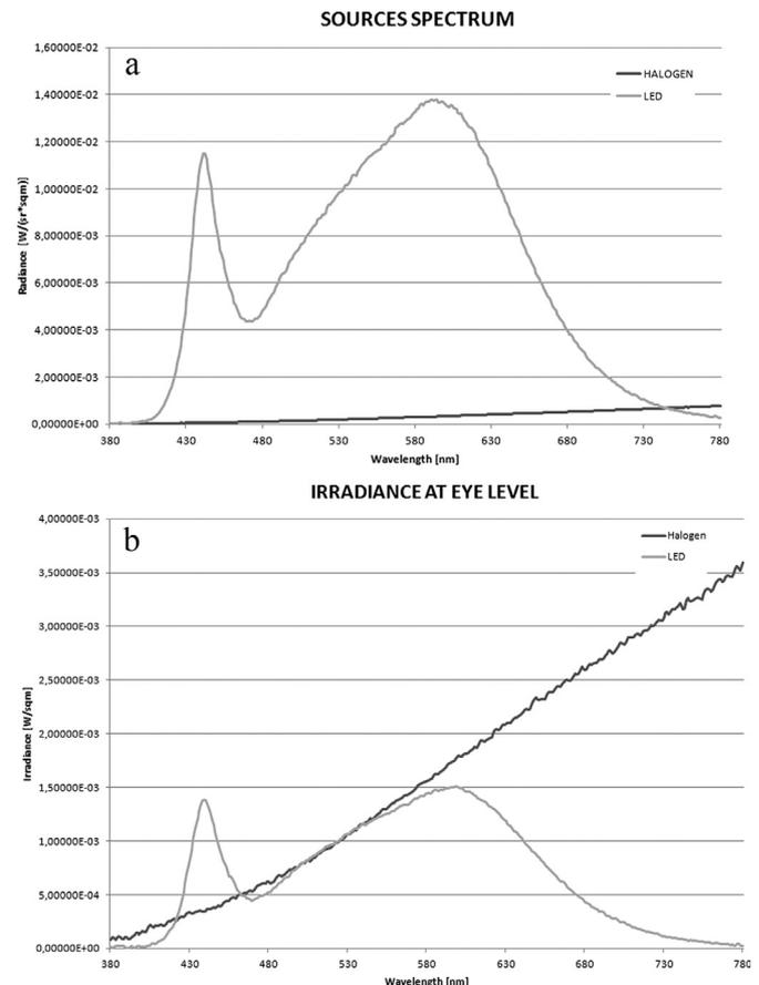
**Fig. 2.** a. Spectrum emitted by halogen lights and LEDs. b. Spectral power distribution of light sources at eye level.
