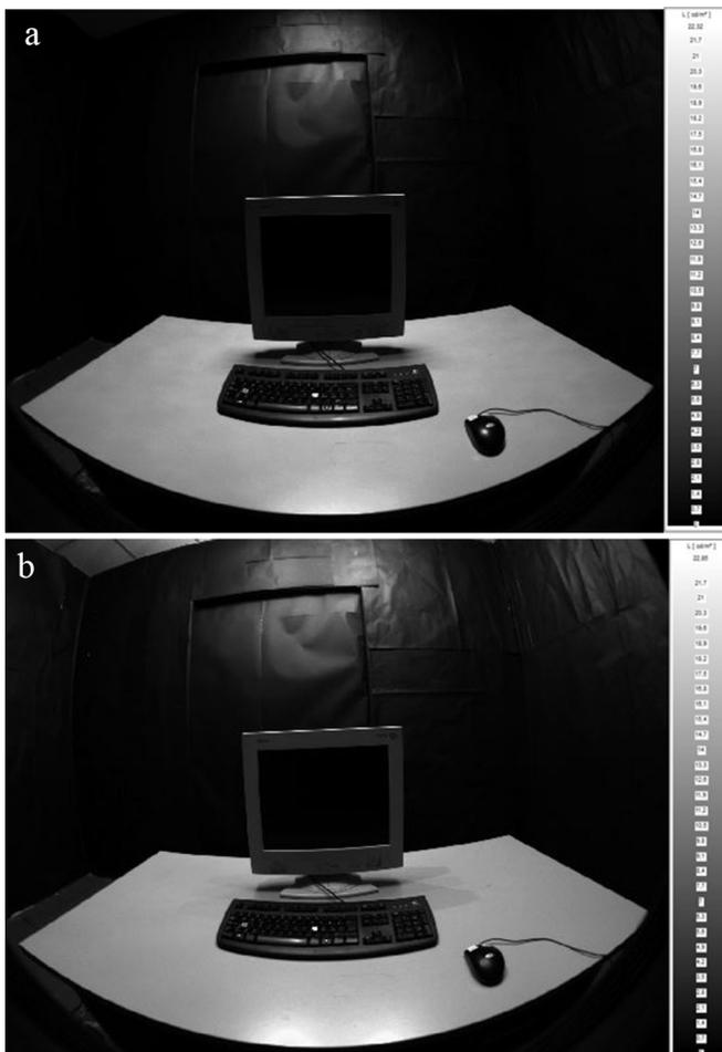
**Fig. 3.** a. Luminance distribution in the visual field with halogen source. b. Luminance distribution in the visual field with LED.
